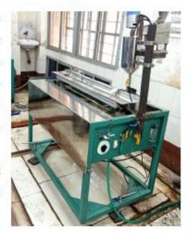
1.5m Drum Scrubber (Batch and continuous) is a custom-designed mineral washer used to remove slime/clay coating from valuable minerals such as iron ore.
